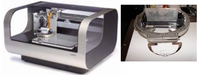
Fig. 3. Material printer DMP-2800 and the print-head DMC-11610.
