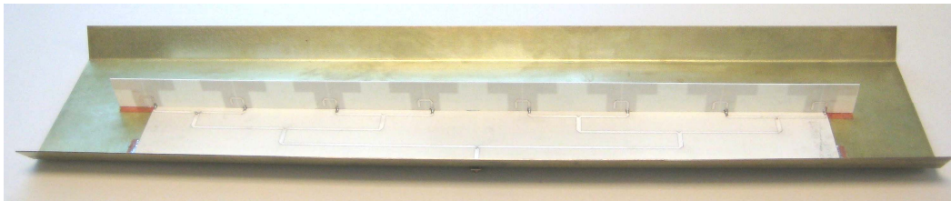
Fig. 4. Eight-element linear array of the printed dipole with adjusted integrated balun.
