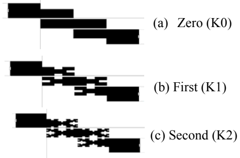
Figure 2 Layout on proposed geometry (1-pole case);K0: zero iteration, K1: the first iteration, K2: the second iteration.
